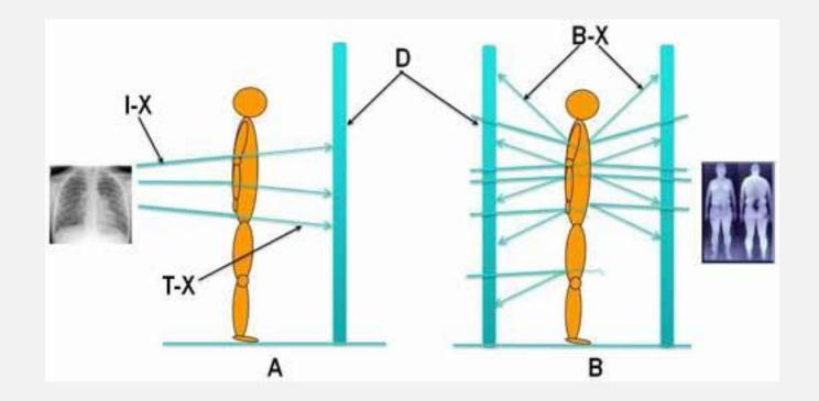
In a backscatter x-ray system, the x-ray intensity is very low and not strong enough to penetrate or transmit through the body, even though a few of the x-rays may be absorbed by the body. However, the majority of the x-rays bounces off or scatters onto the surface. This is the reason for the two large detectors that collect the backscatter or scatter x-rays to create an image.
